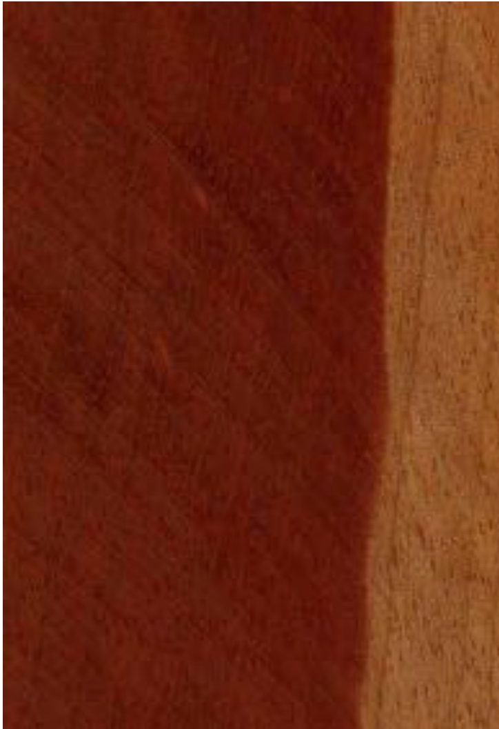
Vivid dark red to reddish yellow Rhengas: Gluta spp. and Melanorrhoea spp. (Anacardiaceae)
