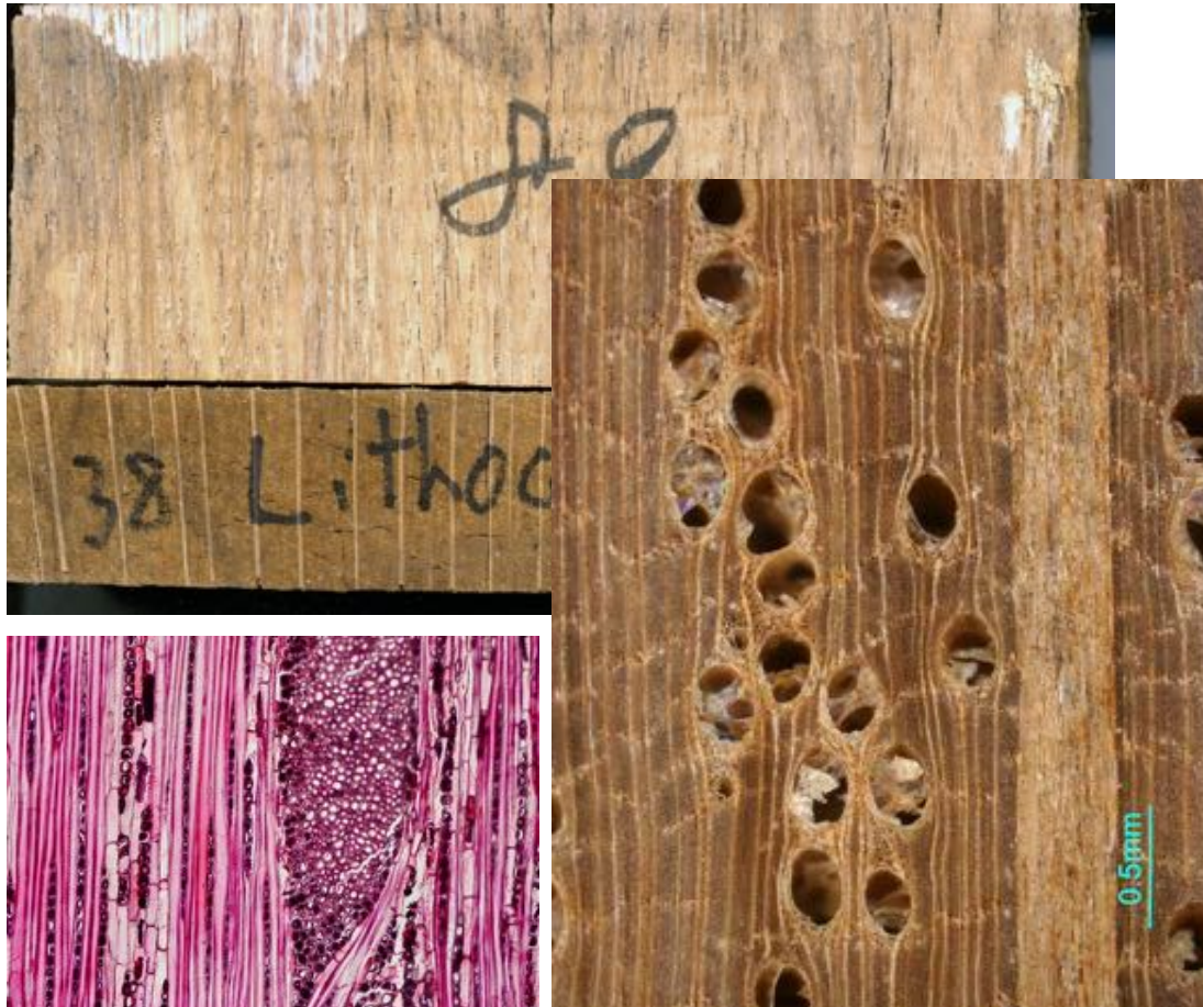
Aggregate of wide rays Mempening: Lithocarpus (or Quercus , Trigonobalanus ) spp. (Fagaceae)
